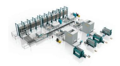
**AJS** is Salvagnini's 4.0 multi-process solution: by combining different production technologies and managing operations via the proprietary OPS software, it schedules, balances and optimizes factory production flows in a completely automatic and flexible manner.
